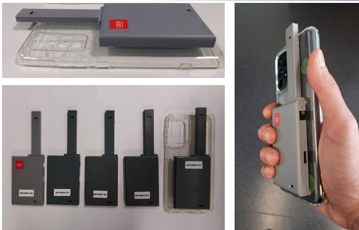
Figure 12. Views of the five full operational DEVIN5G UL-exposimeters (three have been tested by SEAWave partners)
