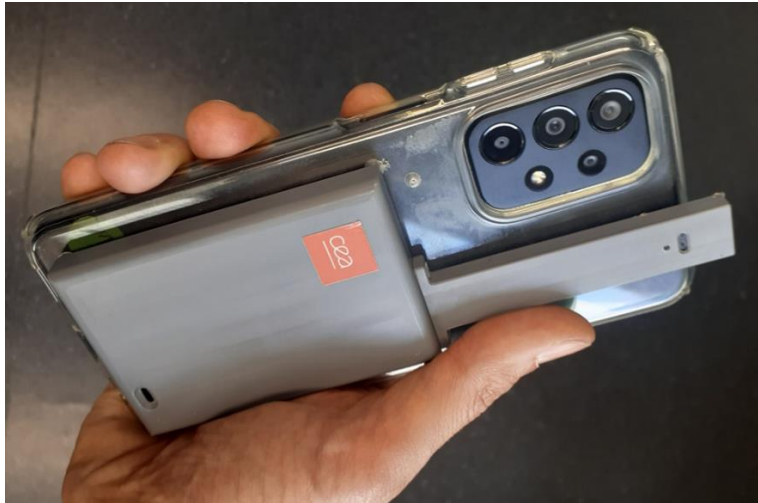
Figure 2. 85 x 55 x 10 mm 3 DEVIN5G instrument mounted on a mobile cover
